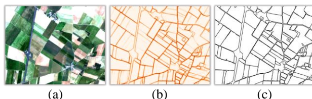
Figure 3 (a) Sentinel-2 RGB image used for field boundary delineation; (b) segmentation result from multi-task DL algorithm; (c) extracted field boundary in vector format.
