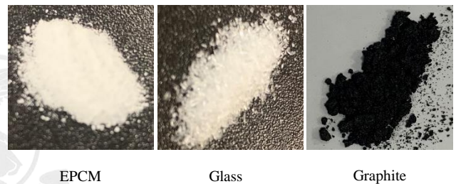
Fig. 1 Materials used for backfilling
