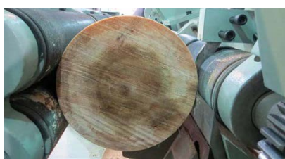
Photo 5: A log being peeled on a spindle-less lathe
