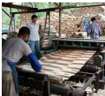
Photo 6: Small scale veneer production in Vietnam showing small diameter logs in the background
